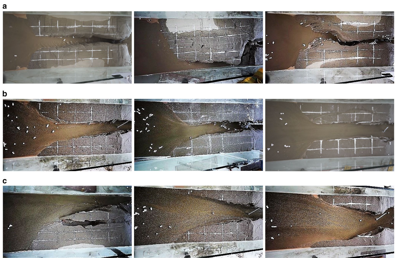
Fig. 5 Comparison of the results of an overtopped dam break a tailings < 0.074 mm in repeated tests; b tailings between 0.074–0.25 mm in repeated tests; c tailings between 0.25–0.5 mm in repeated tests
